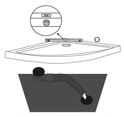
Connect the waste pipe of shower tray to the waste pipe in the floor.
